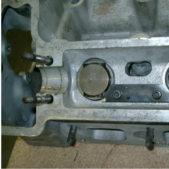
Notched (machined) tappet guides ,the only head work necessary in Gary's design
