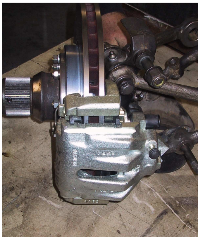
Mounted disc and caliper on Ferrari front end with refurbished bushings, A frame pins, and bearings
