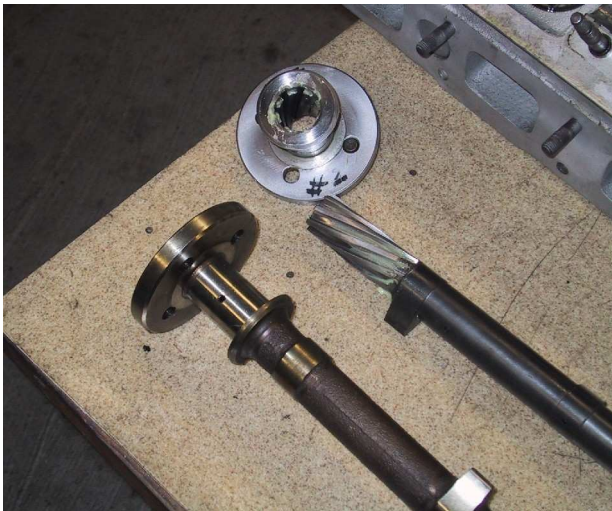
Front cam hub, stock on the bottom and the VVT version with spline on the top
